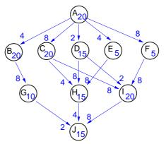
How are the tasks scheduled on the three processors (with HLFET / with ETF)? Draw one Gantt chart for each. Suppose a local communication doesn't cost any time.
